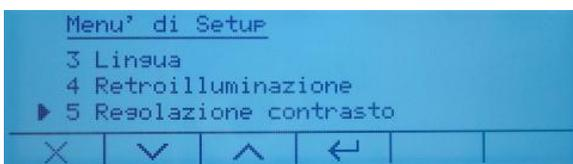
Use the arrow keys
