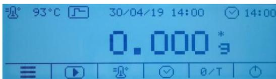
In the weighing screen, the value of the weight loaded on the weighing plate is displayed in the central area.
