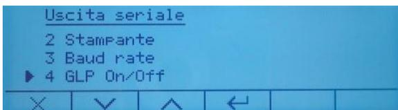
**1 – GLP On/Off:** function that allows you to activate or deactivate the printing of g.l.p. data prior entry by the user.
