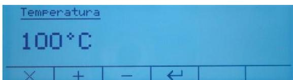
The default temperature is 100°C, so use the keys **+** **-** to increase or decrease the value. Keeping the key pressed for a long time, the value is increased or decreased rapidly.
