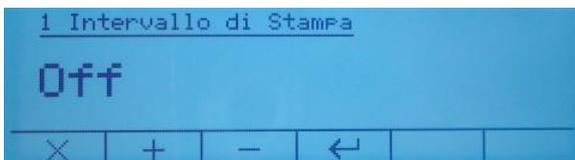
**1 – Print Interval:** this function allows you to define the print interval.
