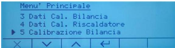
Use the arrow keys
