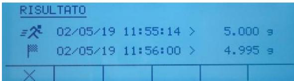
**2. Display the drying result** by pressing the key
