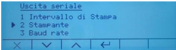
**2 – Printer:** this function allows you to select the device connected to the serial output.
