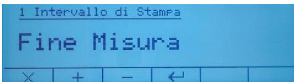
➤ **End Measure**, automatic printing of test results at the end of the analysis.
