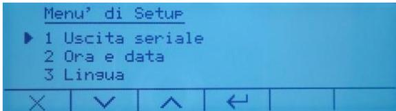
Use the arrow keys
