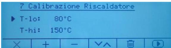
Use the keys **+** **|** **-** to increase and decrease the temperature and the keys **v^** to switch from T-lo to T-hi.
