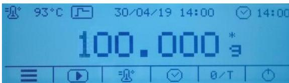
Load the weight or press the key
