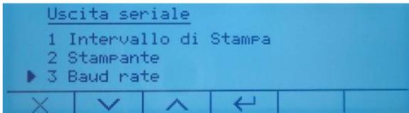
**3 – Baud rate:** parameter for selecting the transmission speed of the serial port.
