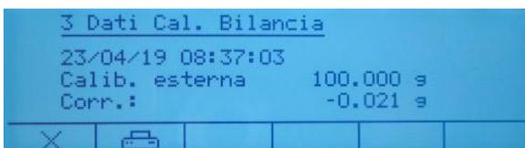
**Calibration Data:** in the calibration data screen, you can check the date on which the last calibration was performed, the mode in which it was performed, the value of the weight used and the correction made with respect to the previous
