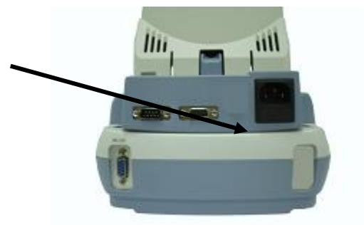
Then connect the VDE cable to the socket located near the device. Do not use cables/extensions that do not comply with current regulations.
