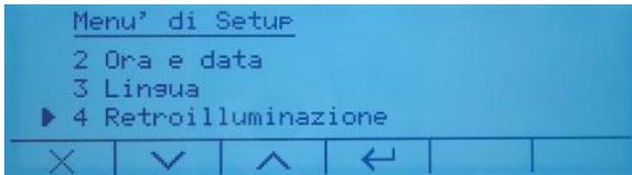
Use the arrow keys
