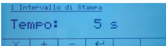
➤ **In Time**, print the analysis data during the test at a set interval. (The settable time interval ranges from 5sec. to 250sec. with 1sec. steps).
