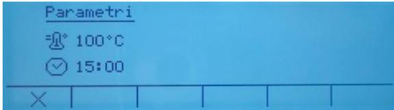
**Parameters:** by pressing the key
