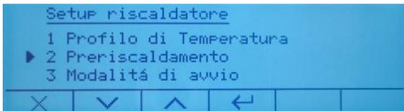
**2 – Warm up:** this function allows you to preheat the heater before performing a drying cycle.
