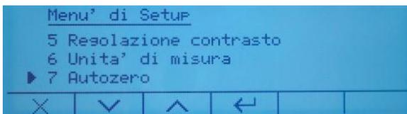
Use the arrow keys
