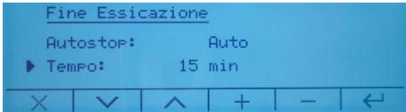
The default cycle time is 15min, so use the keys **+** **|** **-** to increase or decrease the value. Keeping the key pressed for a long time, the value is increased or decreased rapidly.
