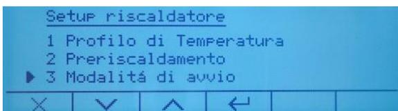
**3 – Startup mode:** this function allows you to choose the mode for starting the drying program.2
