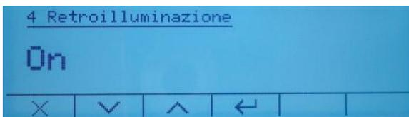
Select the mode with backlighting enabled "On" or disabled "Off" using the up and down arrows.
